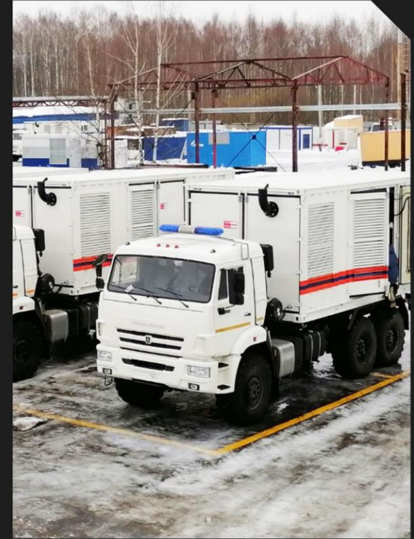
8.5 MW portable electric power plant for Rosseti
